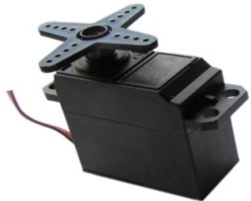
**Similar to the way you used pulses to PWM on LED in the Colour Mixing Lamp Project, servo motors expect a number of pulses that tell them what angle to move to. The pulses always come at the same time intervals, but the width varies between 1000 and 2000 microseconds.**
